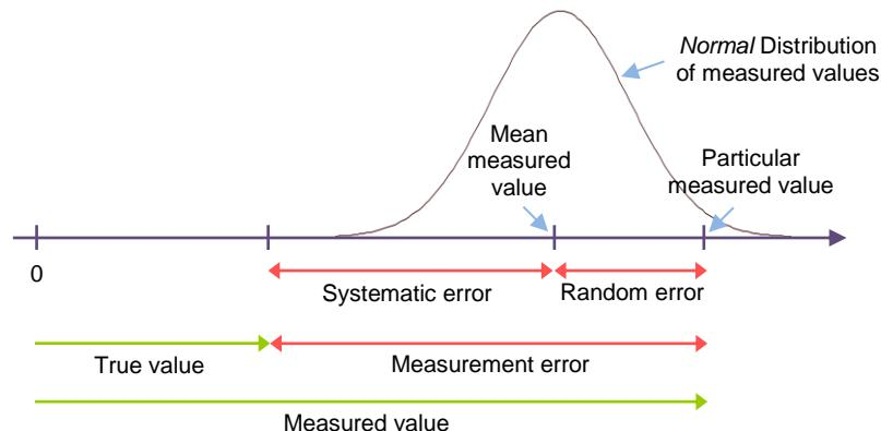
$$\text{Measurement error} = \text{Measured value} - \text{True value}$$
